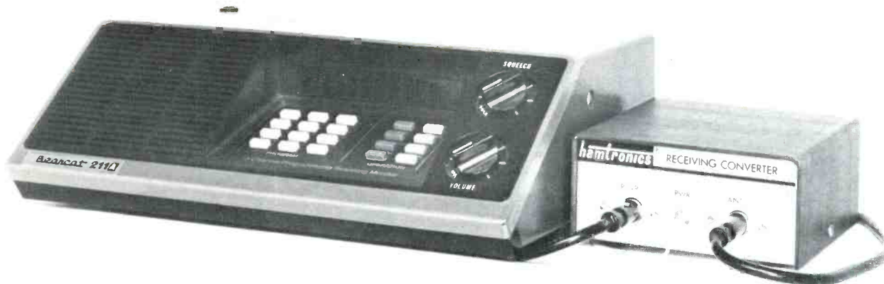
Hamtronics produces a line of converters which can be used with standard band scanners to receive this band.
